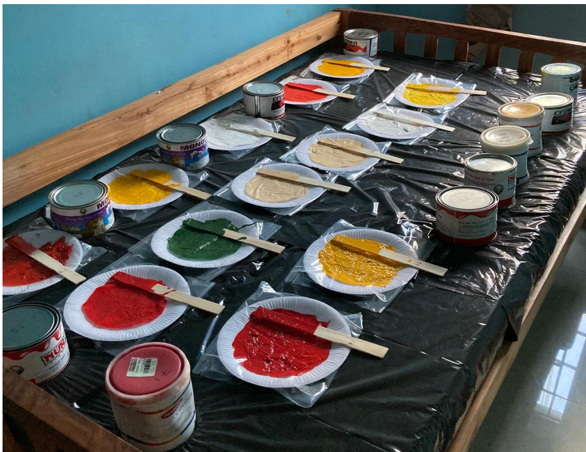
Figure 10 Sample preparation and air drying of paint samples
